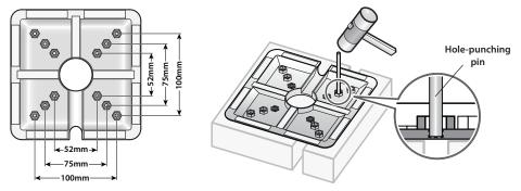
2. Attach the stand using the included screw bolts (4 pcs.) and nuts (4 pcs.). For stand types that are hollow for routing cables through them, at this point perform the routing of the cables through the stand.
