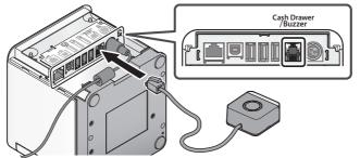
**3.** Connect the cables to suit the location where the device is placed. Plug the power cable to the AC outlet. Turn on the printer. Installation is complete.
