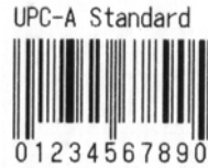
UPC-A Barcode with Guard Bars Extended 2 mm
