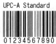
UPC-A Barcode without Guard Bars Extended
